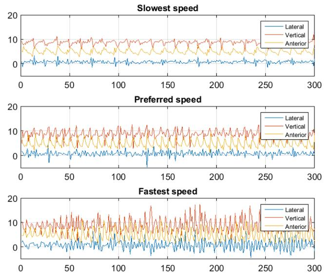
Figure 4. Acceleration from three different gait speeds.
