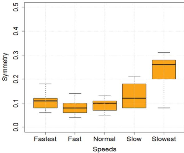
Figure 6. Symmetry result for five different gait speeds.
